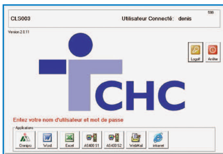
Because medical file security is a very important, CHC has developed a front-end application residing on each WBT that displays the application icons which the user has the right to access via GO-Global. Doctors can access medical files, while clerical staff can only access administrative documents.
